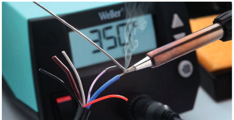
The Weller soldering station includes a 1.6mm 'screwdriver' tip.
